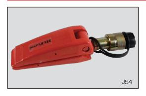
The JS4 hydraulic spreader is the ideal solution for spreading, wedging and prising operations in a wide variety of industrial applications. The compact, low weight, spring assisted return design enables the tool to fit into a gap of 9.7mm and offers a maximum spread of 94mm. Manufactured from high strength steel, with a maximum pressure of 700 Bar, the JS4 is supplied fitted with a quick connect female half coupler, and can be used with HP110 manual hand pump and HC hose.
