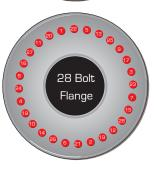
Whether tightening the bolts using a torque wrench or bolt tensioners it is a good idea to carry out a final check for tightness of all the bolts by simply tapping each nut with a hammer and listen to see if a high pitched ringing sound is achieved. A dull sound indicates that the respective bolt is still loose.
