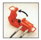
To open the cutter, swivel cutting head forward.
