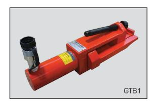
The Hi-Force Giant Bead Breaker is used for breaking tyre beads and suitable for use on 5 piece rims 25" to 51" (635 to 1295 mm). With this model you can remove larger tyres with ease using a powerful 14 tonnes capacity, 700 Bar hydraulic cylinder which has a nett weight of 12.5kgs The Giant bead breaker is compatible for use with Hi-Force 700 Bar hand and powered pumps (see pages 27 - 48).
