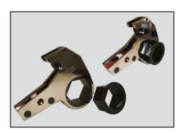
To reduce the female hexagon AF size of the TWH-NRH imperial ratchet heads (see page 77), these Hi-Force hexagon reducer bushes offer an easy and economical solution. Just select your outside AF size (i.e ratchet head AF size) and the required inside AF size to determine the model number. Please note that wall thickness (specified below as 'W' dimension) must be added to the minimum radius dimension of your ratchet head when using a reducer bush.
