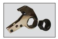
To reduce the female hexagon AF size of the TWH-NRH metric ratchet heads (see page 78), these Hi-Force hexagon reducer bushes offer an easy and economical solution. Just select your outside AF size (i.e ratchet head AF size) and the required inside AF size to determine the model number. Please note that wall thickness (specified below as 'W' dimension) must be added to the minimum radius dimension of your ratchet head when using a reducer bush.
