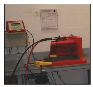
Additionally, torque equipment is calibrated, using the latest technology. Test & calibration results are automatically transferred to purpose-written software for producing unique and traceable certificates.
