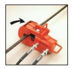
Step 3: Close the cutting head by swivelling it back to its original position and secure behind the latch.
