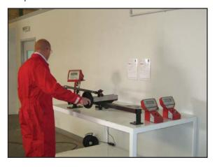
Hydraulic torque wrench calibration
