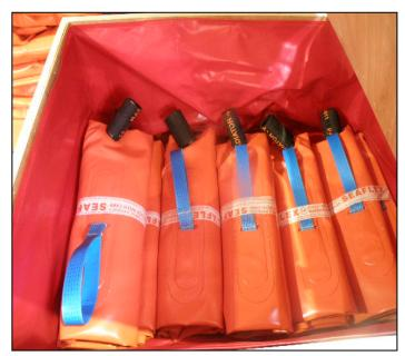
Pump, hoses and manifold in one side of transit case 375kg Test Weights in opposite side of transit case.
