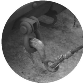
Proper hook placement for lifting and lashing vehicles.
