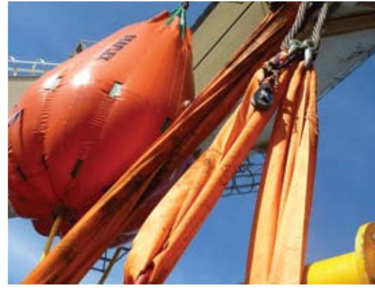
Made from High Tensile Trevira® Polyester 3/3, coated with heavy duty UV stabilised PVC coating, and with integrated slings and fittings which comply with relevant British Standards and LEEA guidelines, our WaterLoad test weights are built to last. High quality performance, robust fabrics, reliable RF welded seams and versatile filling/ discharge arrangements have made Seaflex WaterLoad bags the first choice for an ever-increasing numbers of test houses around the world.
