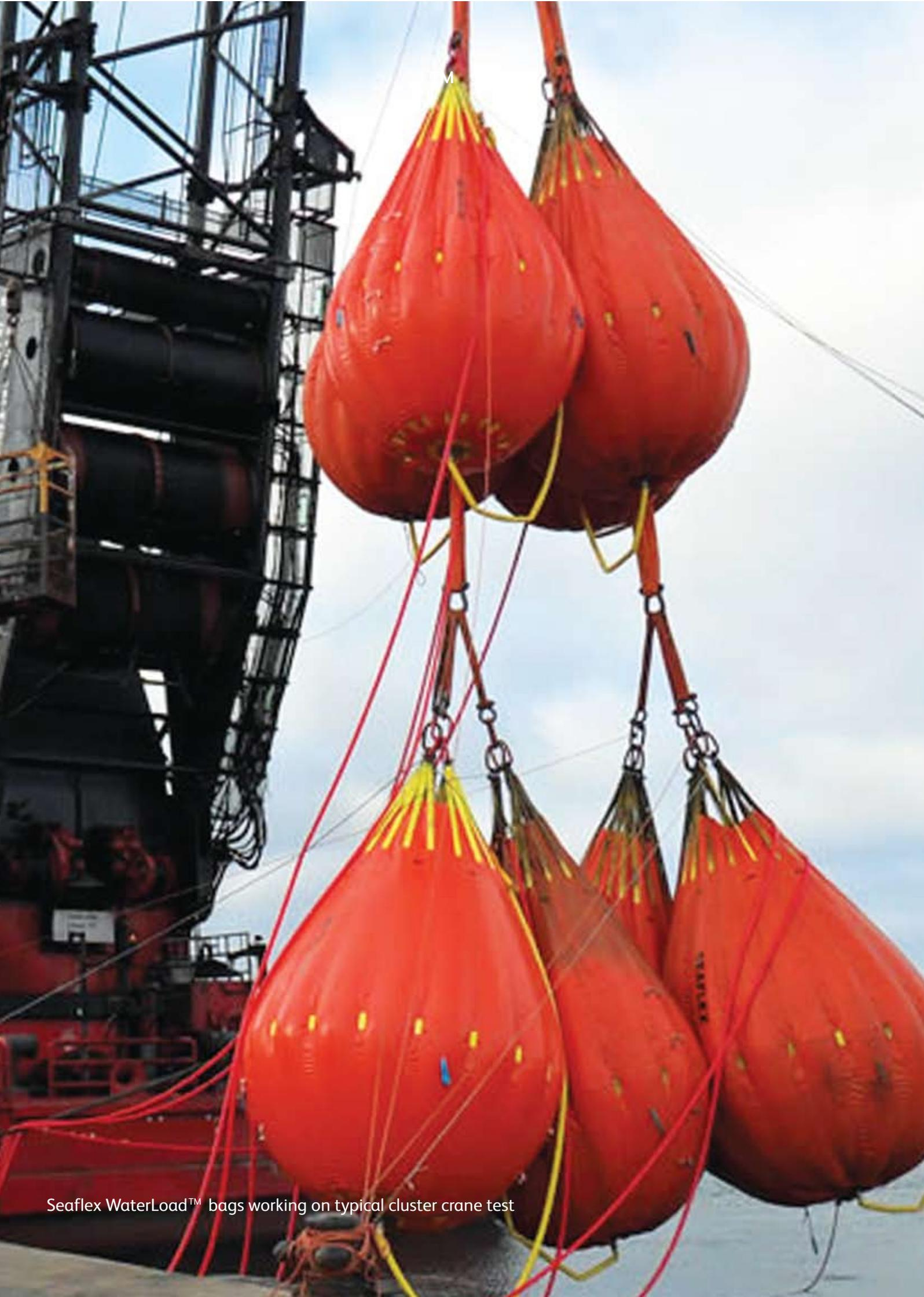
Seaflex WaterLoad™ bags working on typical cluster crane test
