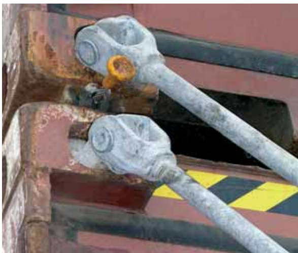
SECURING WITH PARALLEL LASHING RODS AND SEMI-AUTOMATIC TWISTLOCK
